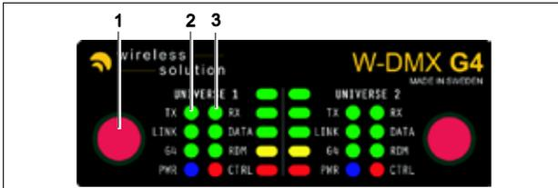
2. Press and hold the left red function button (1) on the front panel (Universe 1).
