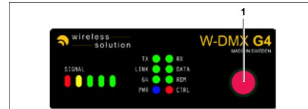
2. Press and hold the red function button (1) on the front panel.
