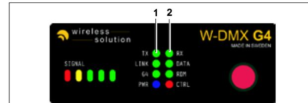
→ The mode is switched. The LEDs indicate the current mode: either TX (1) or RX (2):
