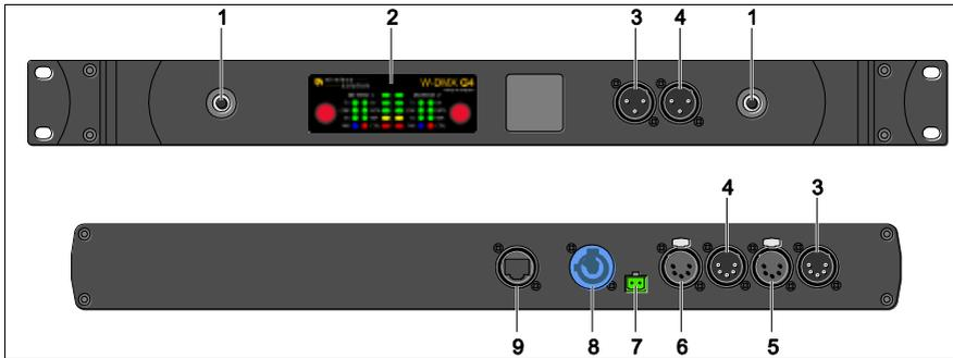
Fig. 16: Connectors and ports of ProBox F-2500
