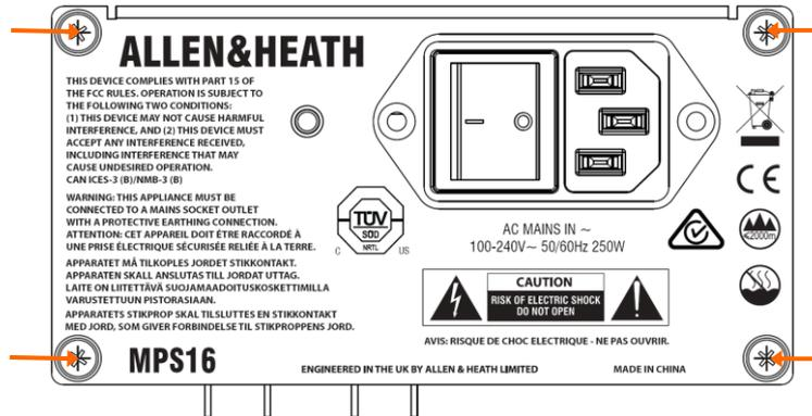
**i** dLive Surfaces ship with one PSU fitted. A second PSU can be fitted for redundancy (part number MPS-16). Loosen the 4 captive thumb screws securing the blank panel\*, slide the PSU into the slot, and tighten the 4 captive thumb screws indicated above. The Surface will automatically switch between the supplies without interruption to the audio should one fail.
