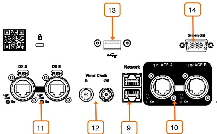
**9 Network** – 2 RJ45 Gigabit Ethernet ports. Connect a laptop or a wireless router to use with dLive Editor or iOS apps. All devices on the network must have compatible IP addresses.
