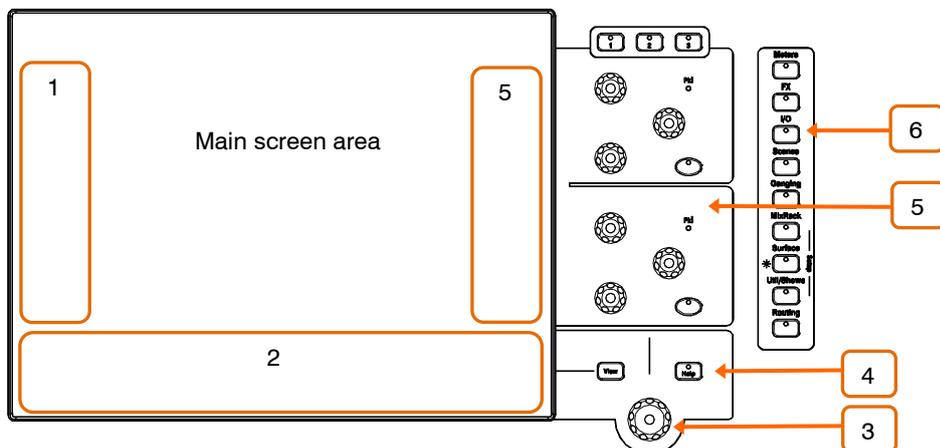
**1** **Left widget area** – Can be configured for different functions, for example as a scrollable Scenes list. Hold down **Setup** and touch this area to configure.
