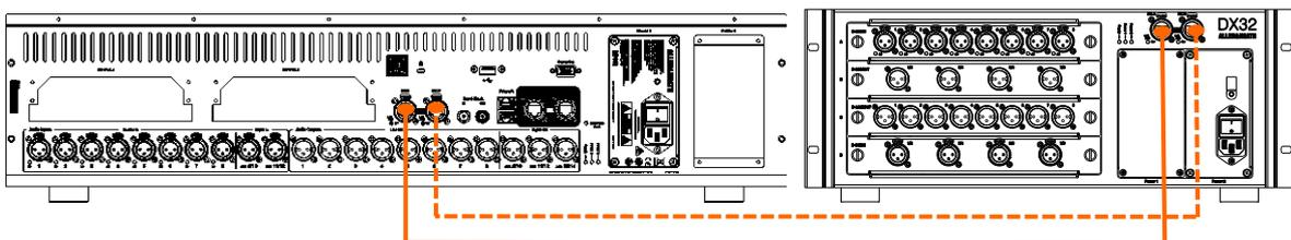
Switch on the DX Expander. The DX port Lnk/Err indicators flash at a steady rate when the link is established. The red error indicator lights if a communication error is detected. Check that the cables are correctly plugged in and are not faulty.
