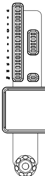
**Meter** – 22-segment signal meter and 6-segment gain reduction meter. The meter displays audio signal activity for the channel.
