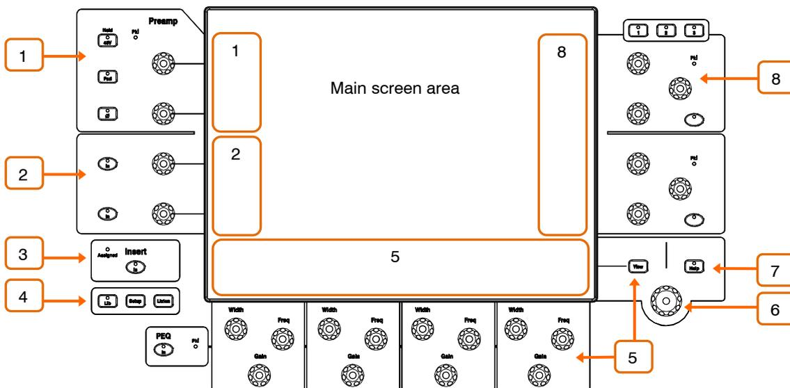
1 **Preamp** – Peak indicator and dedicated preamp controls for analogue Gain, Digital Trim, 48V, Pad and polarity.
