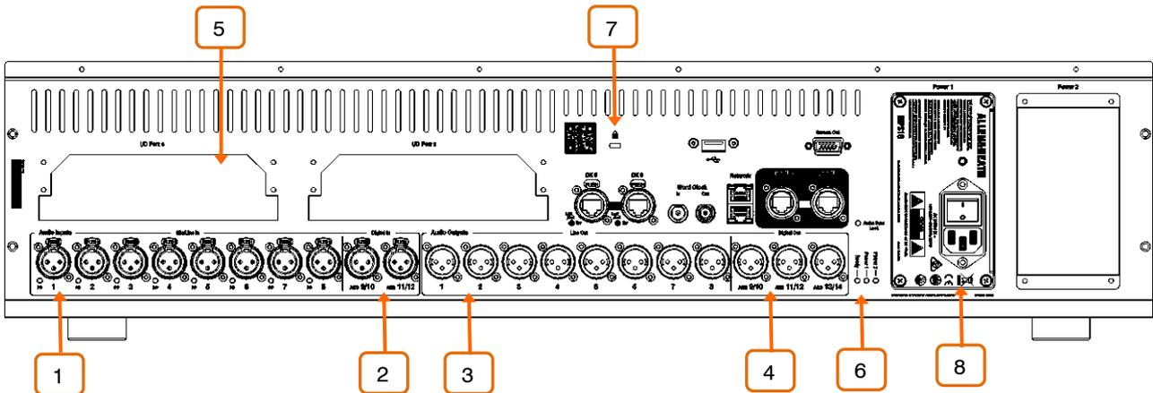
**1 Mic/Line inputs** – 8x recallable preamps for balanced or unbalanced microphone and line level signals. Gain, Pad and 48V are digitally controlled within the preamp.
