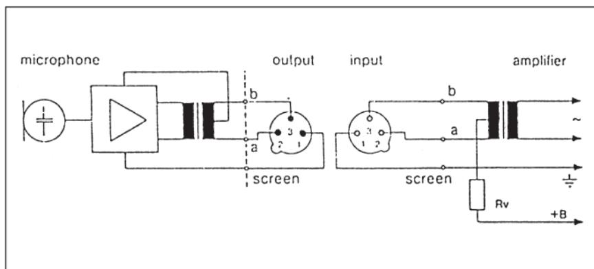
Input circuitry incorporating transformer **without** center tap (ungrounded).
