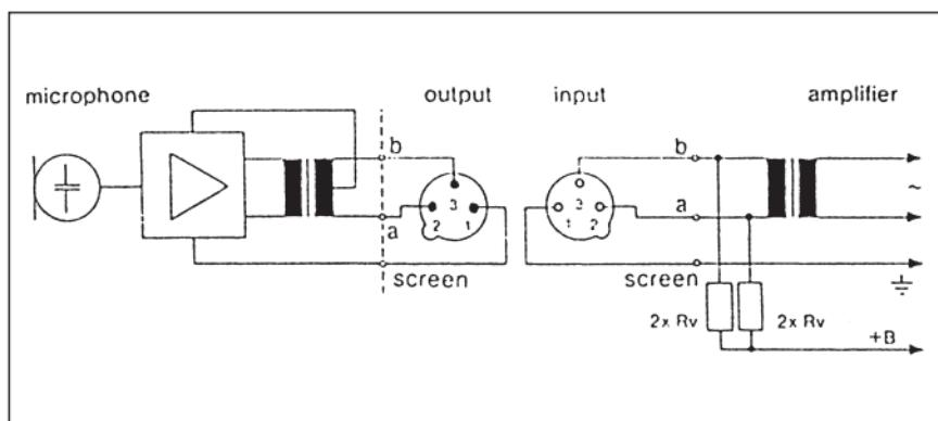
The resistors  $2 \times R_v$  must have a tolerance not exceeding 0.5 % in order to satisfy the symmetry requirement.
