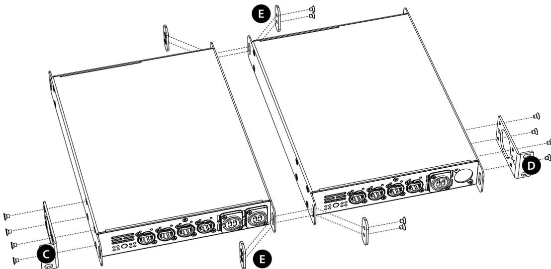
To combine a GigaCore 10 device with a Luminex half 19" device, style LumiNode 4, the mounting procedure differs a little. The bolt (F), not included, replaces the rear couplers at the rear side of the devices. Use the correct bolt, M10x20, with a screw wire no longer as 20mm. You can order this part from Luminex (Part Number: R 90 01042)
