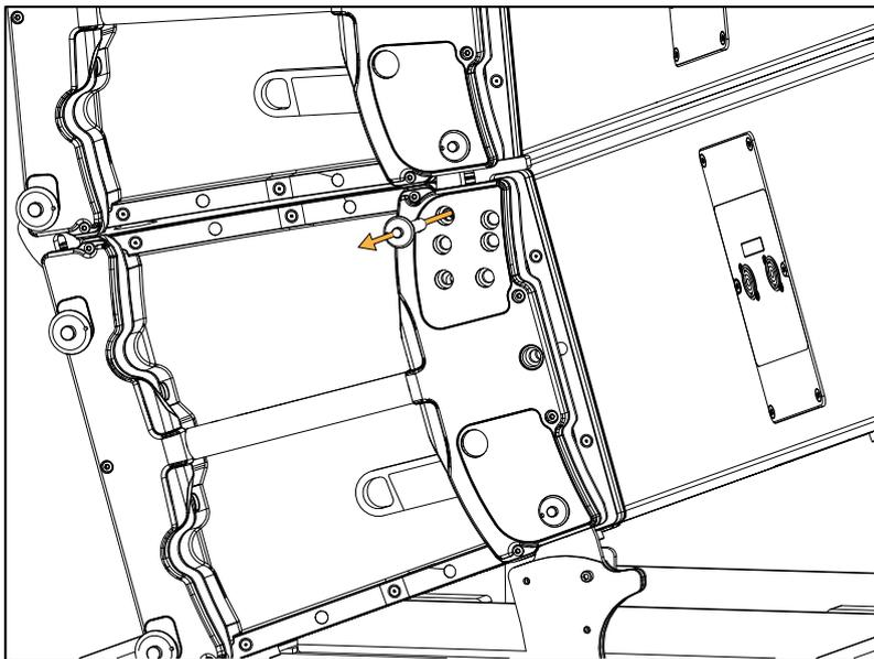
2. Position the pin at the chosen angle hole and slide the rigging arm until the pin goes in.
