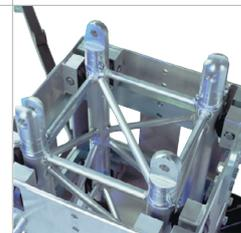
4 A completely mounted hinge set. First locate the hinge pins on one side. The truss now works as a hinge and can be erected easily. Subsequently locate the remaining hinge pins in the other side to fix the mast into position. Per tower 4 x CCS6-H needed. (hinge set MPT-ST tower).
