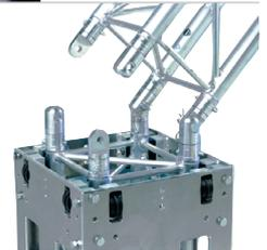
5 Unscrew the screw jacks in the outriggers. Make sure that the castors of the base are free of any load. The complete load of the base should be supported by the screw jacks. Level the base by adjusting the screw jacks. The base must be perfectly level before the mast is erected. Long outriggers are needed for structures with three towers or less. Make sure the screw jacks can absorb tower forces through filler plates where needed.
