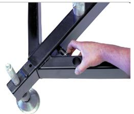
3 Disassemble the hinge set, mount the half hinges to both the mast sections (H30V truss). Male and female connections should be mounted diagonally (as shown in the picture) in order to facilitate the erection of the mast.
