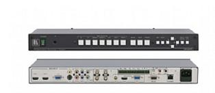
The VP-437xl is a 7-input scaler/switcher for composite (Y/C), video, s-Video component video, computer graphics video and HDMI with unbalanced stereo and S/PDIF audio signals. It scales the selected video signal to computer а graphics or HDTV output resolution, embeds the audio and outputs an HDMI signal. The VP-437xl is the same as the VP-436 with the addition of Ethernet control
