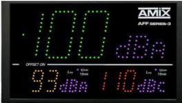
*LAeq has exceeded the first threshold and the LCeq has exceeded the second configurable threshold.*
