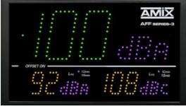
*LAeq and LCeq have exceeded the first threshold*
