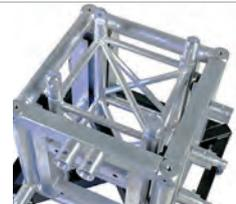
**5** A completely mounted hinge set. First locate the hinge pins on one side. The truss now works as a hinge and can be erected easily. Then locate the remaining hinge pins on the other side to fix the mast into position. Per tower 4 x CCS6-H are needed (hinge set MPT•ST tower). Only use CCS-604ST spigot pints to connect the mast sections, to prevent damage to your sleeve block and the risk of getting "stuck".
