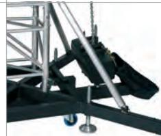
**4** Disassemble the hinge set, mount the half hinges to both mast sections (S40T truss). Male and female connections should be mounted diagonally (as shown in the picture), in order to facilitate the erection of the mast.
