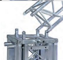
**6** Unscrew the screw jacks in the outriggers, making sure that the castors of the base are free of any load. The complete load of the base should be supported by the screw jacks. Level the base by adjusting the screw jacks. The base must be perfectly level before the mast is erected. Long outriggers are needed for structures with three towers or less.
